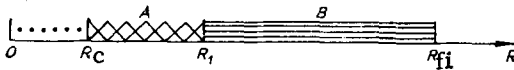
Fig. 1. Schematic representation of the different zones in a medium after an explosion when there is no slit. Cavity ( R \geq R_C ): A) crushing zone ( R_C \leq R \leq R_1 ); B) radial fissure zone ( R_1 \leq R \leq R_{fi} ).
